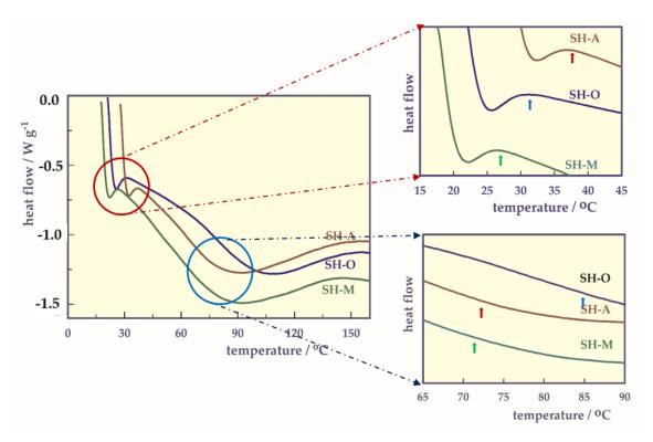
Figure 5. DSC thermograms of the hydrogels.
