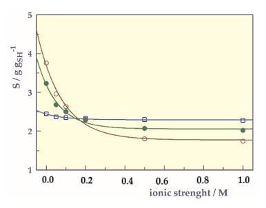
Figure 8. Ionic strength-responsive swelling of SHs,  $\Box$ ; SH-O, o; SH-A,  $\bullet$ ; SH-M, and —; model fit.
