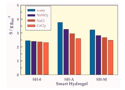
Figure 9. Ion and counter ion-dependent swelling bar graph of SHs.
