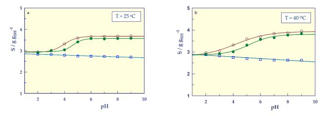
Figure 6. pH-responsive swelling of the SHs at 25 <sup>O</sup>C (a) and at 40 <sup>O</sup>C (b), □; SH-O, o; SH-A, •; SH-M, and --; model fit.
