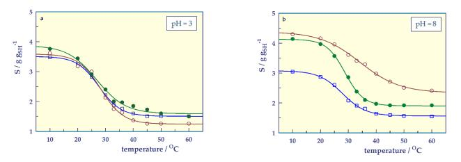
**Figure 7.** Temperature-responsive swelling of the SHs at pH = 3 (**a**) and at pH = 8 (**b**),  $\Box$ ; SH-O, o; SH-A, •; SH-M, and —-; model fit.
