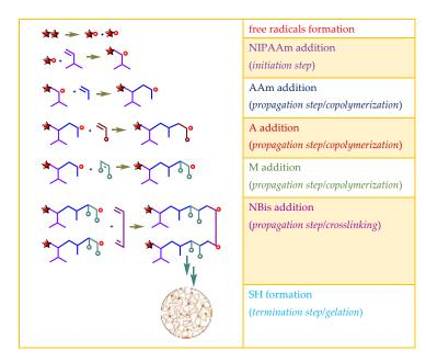
Figure 1. The plausible polymerization and crosslinking mechanism of the hydrogels.
