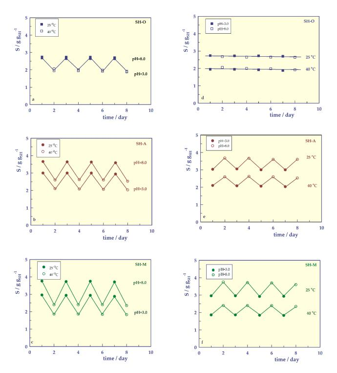
**Figure 11.** Temperature-responsive reversible swelling profiles of SHs at pH = 3 and at pH = 8; (a) SH-O, (b) SH-A, (c) SH-M, and pH-responsive reversible swelling profiles of SHs at 25 °C and at 25°; (d) SH-O, (e) SH-A, (f) SH-M.
