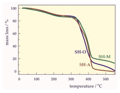
Figure 3. TG thermograms of the hydrogels.
