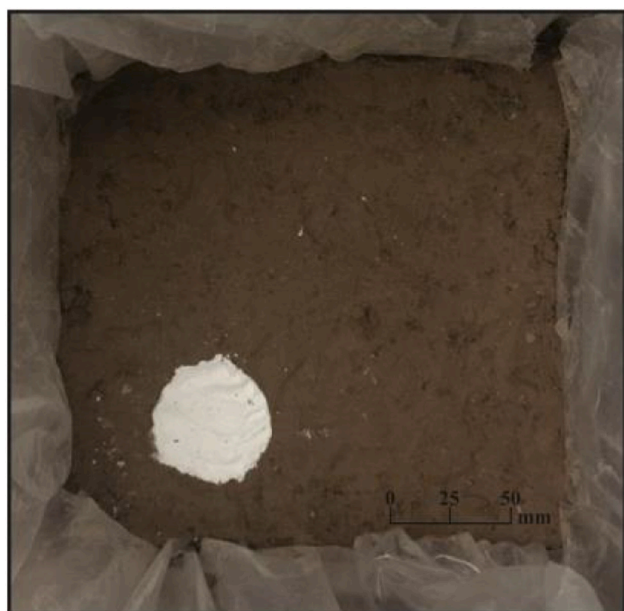
Fig. 8. The top view of a typical model designed for the column performances of the additives.
