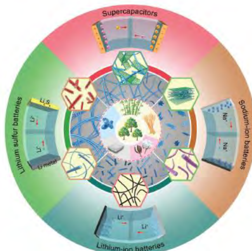
Figure 1. A schematic representation showing the use of nanocellulose to energy storage applications [5].
