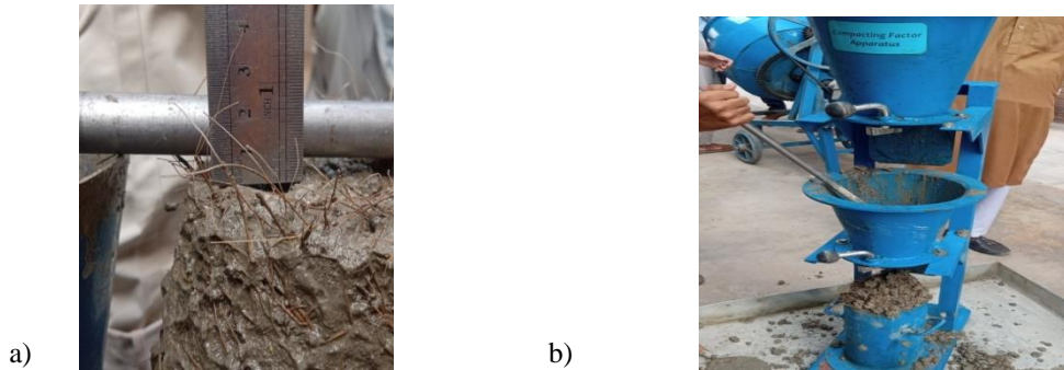
Figure 1: Workability tests, a. slump, and b. compaction factor
