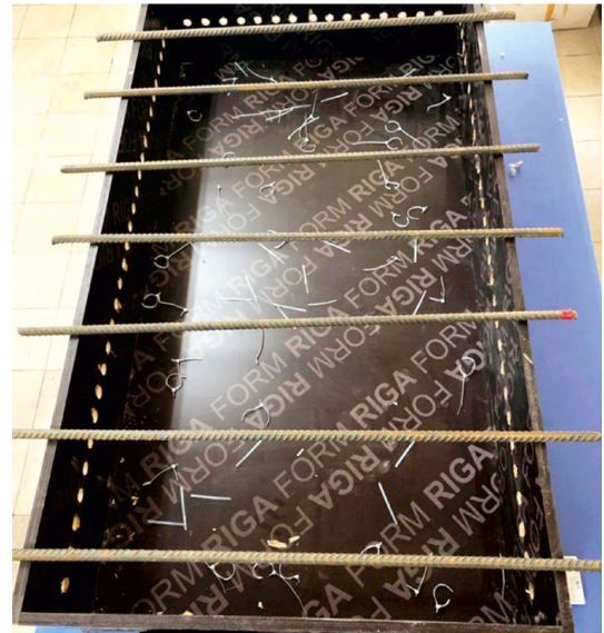
FIGURE 11. Locations of the construction steel placed in the third test system with the size of 80 × 150 cm.
