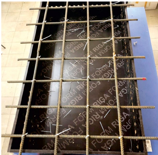
FIGURE 14. Locations of the construction steel placed in the fourth test system with the size of 80 \times 150 cm.
