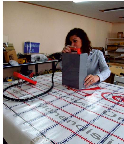
FIGURE 12. MFL measurement performed on the third test system with the size of 80 × 150 cm.
