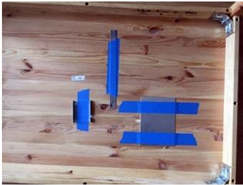
FIGURE 9. Locations of ferromagnetic materials placed in the second test system with the size of 85 × 50 cm (bottom view).
