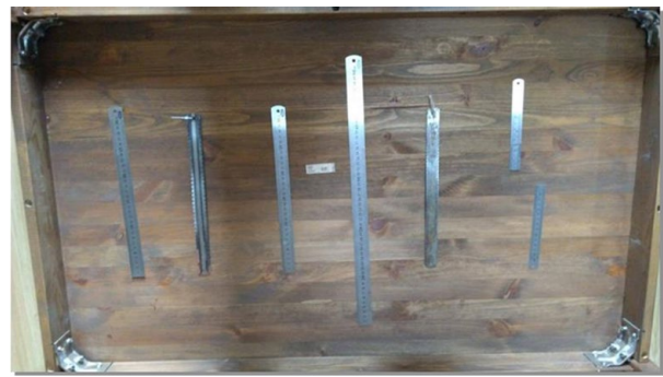
FIGURE 6. Locations of ferromagnetic materials placed in the first test system with the size of 90 \times 60 cm (bottom view).
