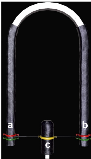
FIGURE 3. Receiver and transmitter coils (a) transmitter 1 (b) transmitter 2 (c) receiver (first prototype).
