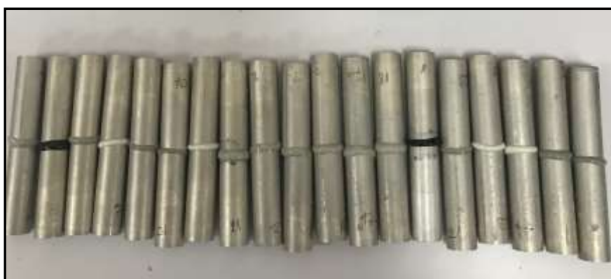
Figure 3: Examples of adhesive-joined butt joint samples.
