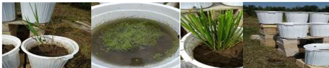
Fig.1. Planting plants inside wetlands and placing wetlands on platforms
