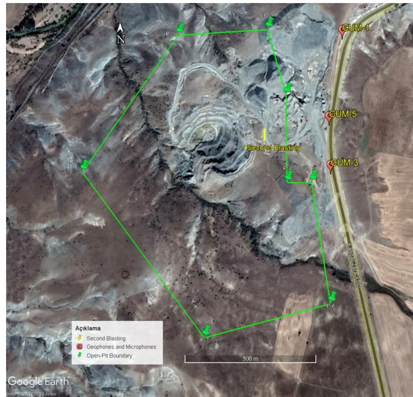
Figure 7. Measurement points of ground vibration and air blast (Second blasting).
