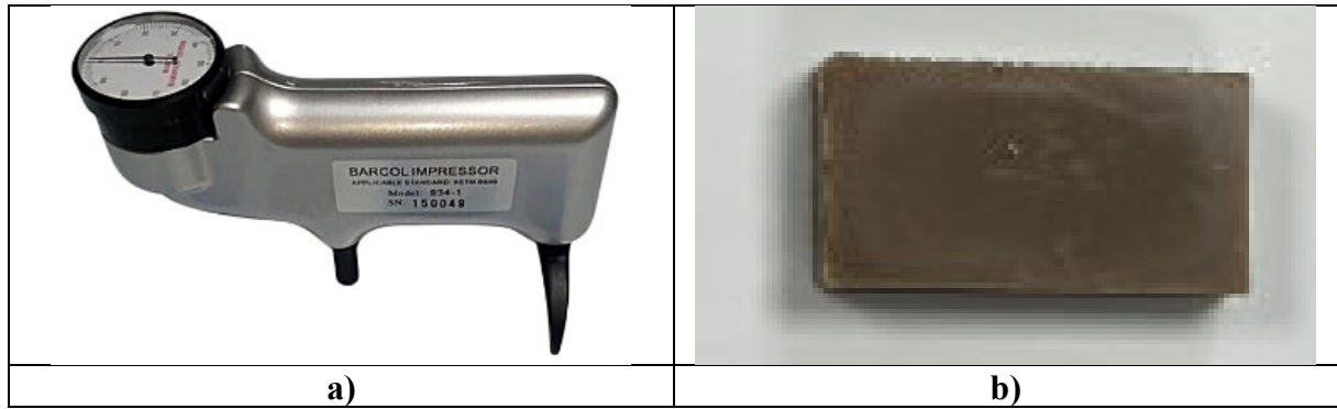
Figure 4. a) hardness measuring device used in the experiments b) test specimen
