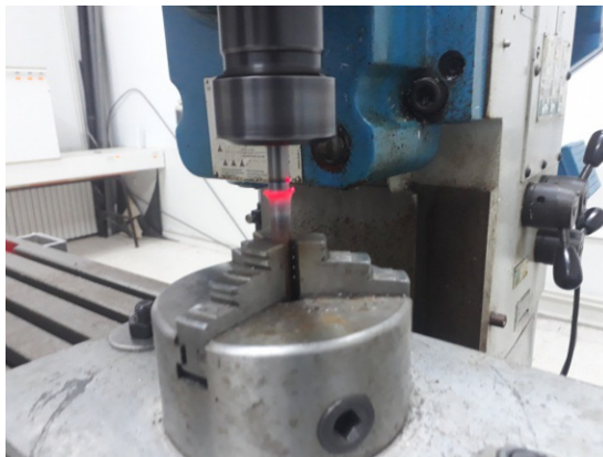
Fig.5. Friction welding of copper bar to A60 steel bar, carried out on a universal milling machine.
