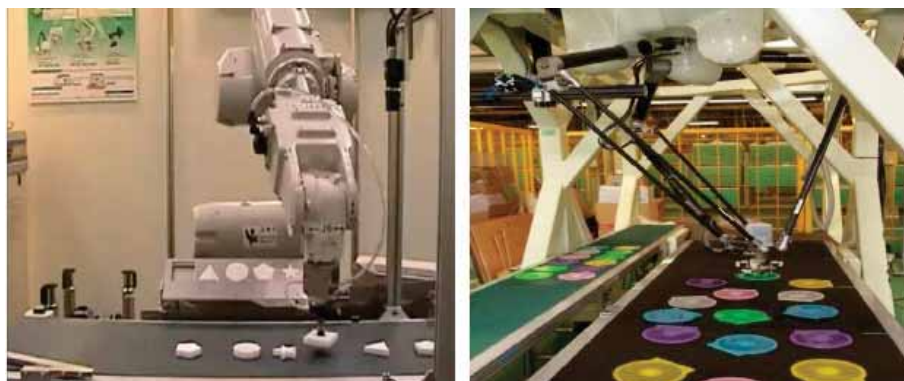
FIGURE 1 Visual sorting robot on the assembly line.
