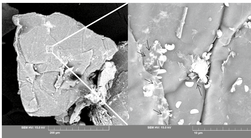
Fig. 5 SEM images of uranyl adsorbed Ch–V composite. \{[\text{UO}_2^{2+}]_0: 1000 \text{ mg L}^{-1}, \text{ adsorbent dosage: } 100 \text{ mg, V: } 10 \text{ mL, natural pH: } 4.0\text{--}4.5, \text{ contact time: } 24 \text{ h, temperature: } 25 \text{ }^\circ\text{C}\}
