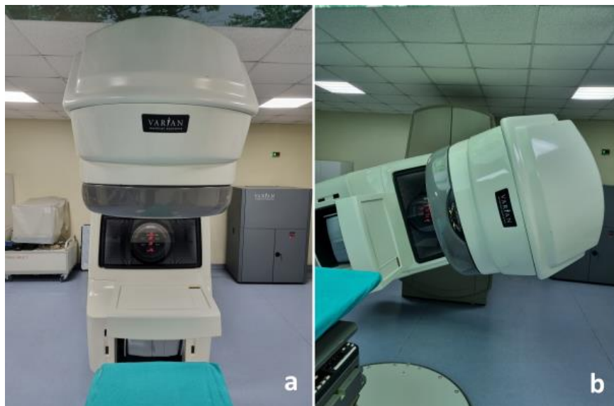
Figure 1 – Experiment set-up: pretreatment verification with fixed gantry angle (a), pretreatment verification with non-fixed gantry angle (b)
