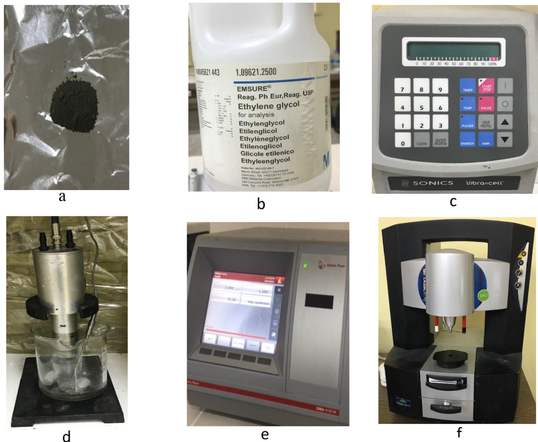
Fig. 1. Figures of rGO-Fe 3 O 4 -TiO 2 nanoparticles (a), EG (b), Sonics VCX-750 Probe Sonicator (c-d), Density meter: DMA 4100 M (e), Malvern Kinexus Pro, UK Stress Controlled Rheometer (f).
