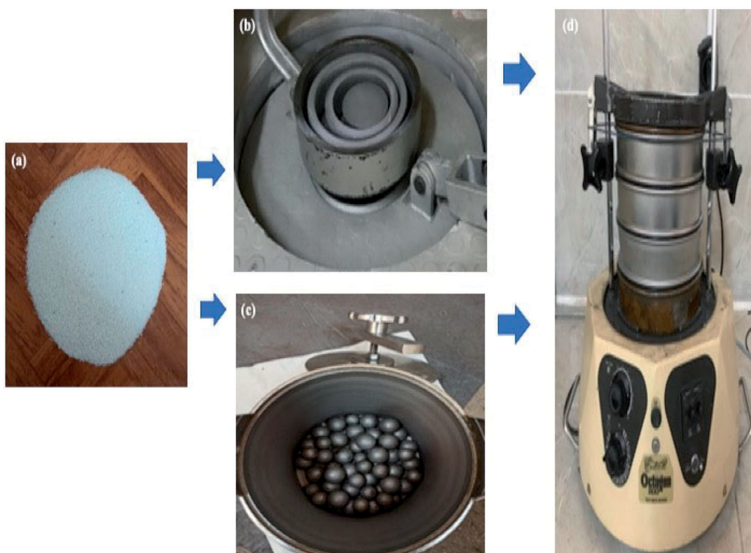
Figure 3. (a) Quartz sample prepared as 0.600–0.850 mm size fraction (b) ball mill (c) vibratory disc mill (d) sieving shaker used for the sample preparation.
