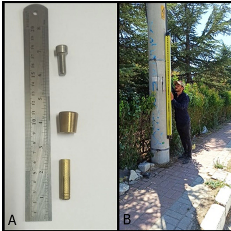
Figure 4. A) Installed benchmarks and B) utility poles where the benchmarks were installed.
