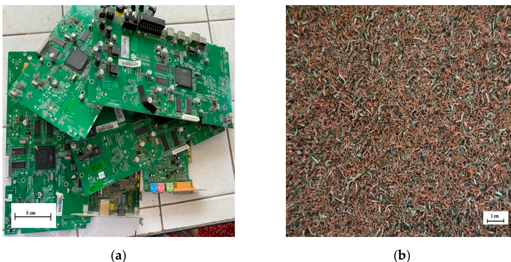
Figure 1. The samples used in experimental studies: (a) EOL PCBs and (b) WEWs.
