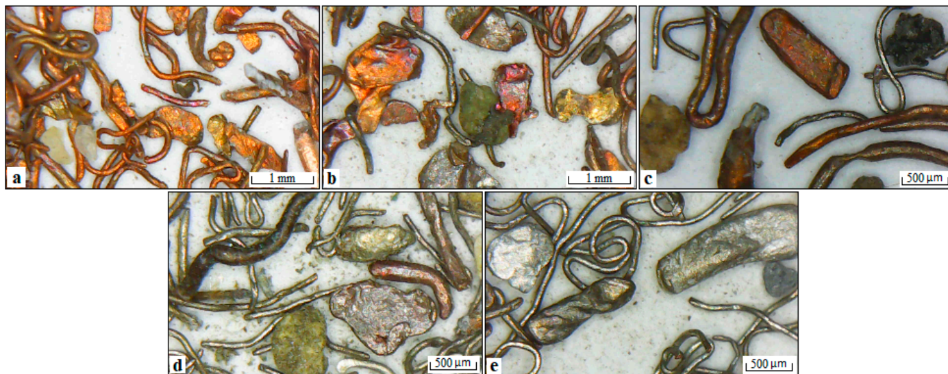
Figure 10. Optical micrographs of the particles in the float ((a): float 1; (b): float 2; (c): float 3; (d): float 4) and the sink (e) fractions after the flotation test.
