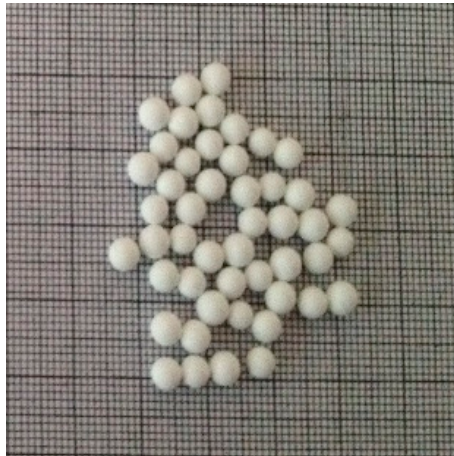
Figure 5. Grinding media used in this study (a) alumina balls used for stirred mill grinding, (b) cylpebs used for ball milling tests [40].
