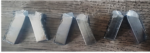
Figure 14: Fractured specimens after notch impact test.
