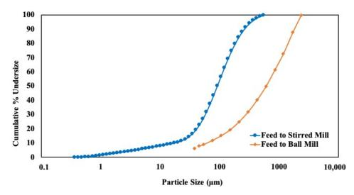
**Figure 3.** Particle size distributions of feed for calcite grinding by the stirred mill and ball mill (modified from [39,40].
