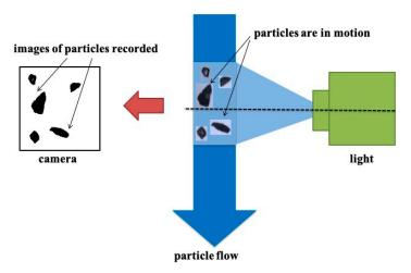
Figure 6. Principle of dynamic imaging of particles.
