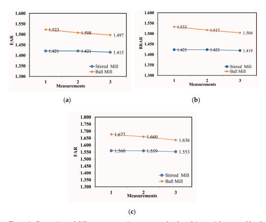
**Figure 9.** Comparison of different aspect ratio parameters for the calcite particles ground by the stirred mill and ball mill by dynamic image analysis: (a) EAR (b) BRAR and (c) FAR.
