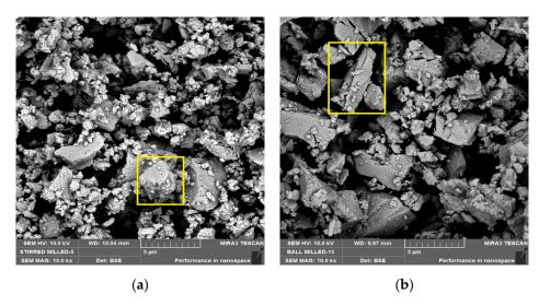
Figure 11. SEM micrographs of the (a) particles from the stirred mill and (b) particles from the ball mill (magnified at  $10,000 \times$ ).
