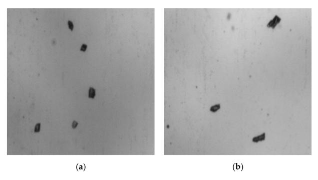
**Figure 10.** Images recorded during DIA measurement (**a**) particles produced by the stirred mill and (**b**) particles produced by the ball mill.
