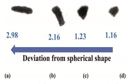
**Figure 2.** Variation of different BRAR values measured by DIA for different shapes of calcite particles. (a) very high BRAR (b) high BRAR (c) moderate BRAR (d) very low BRAR.
