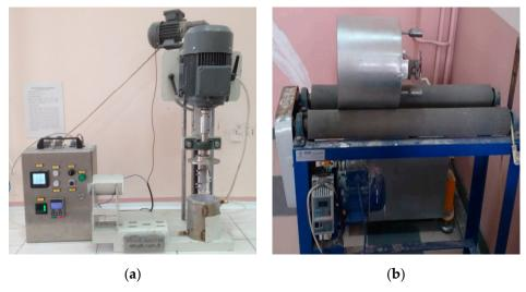
Figure 4. Mills used in this study (a) stirred mill [39], (b) ball mill [40].
