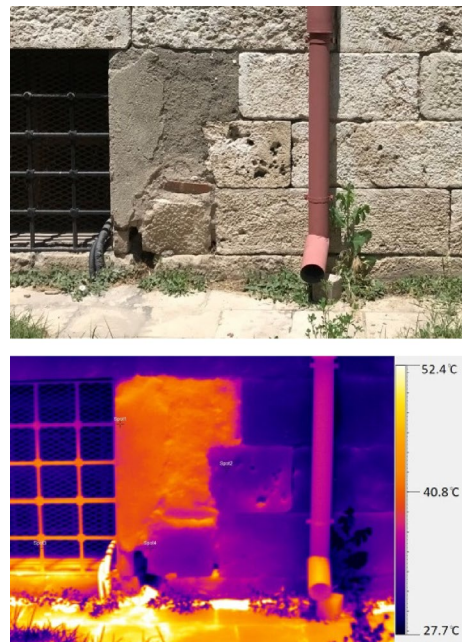
Fig. 17 Detection of plant growth and material differences with the thermal camera
