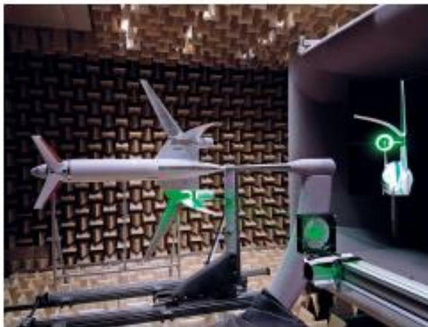
Figure 3. Top view of a scale model of DLR's Low Noise Aircraft in the Low-speed wind tunnel Braunschweig (NWB) operated by the foundation Deutsch-Niederländischer Windkanal (DNW) (German Aerospace Center (DLR) 2019).
