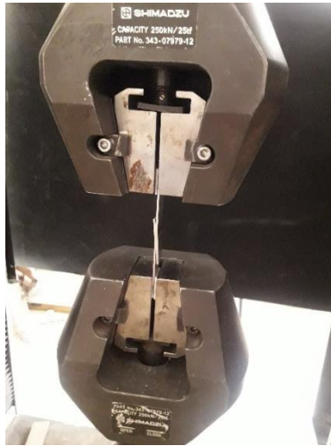
Figure 4. Tensile testing the welded specimens
