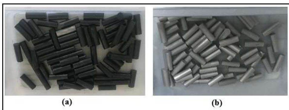
Figure 1: Removing the oxide layer from the surface of aluminum parts, a) aluminum parts after removal of the oxide layer, b) aluminum parts with NaOH solution removed.
