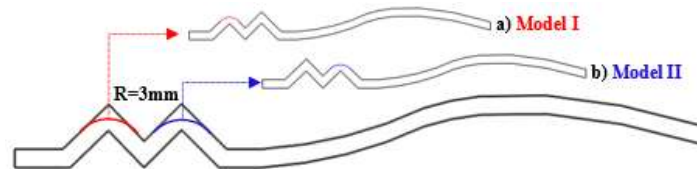
Figure 2. Schematic view of a) first peak rounded (Model I) and b) second peak rounded (Model II) corrugated B airfoils
