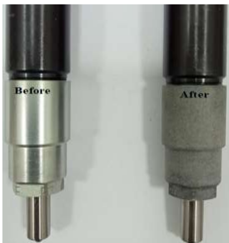
Figure 14. The corrosion effect of ammonium hydroxide on the fuel injector.
