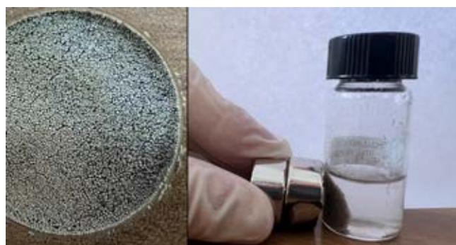
Magnetic properties and shape of PLA@CNTs nano-particles
