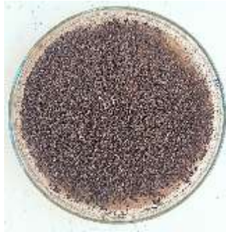
Figure 2. The photograph of SBP-incorporated Fe 3 O 4 nanoparticles after synthesis
